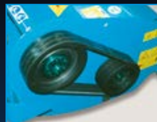
Trasmissione con RL e cinghie dentate Free wheel and toothed belts transmission
