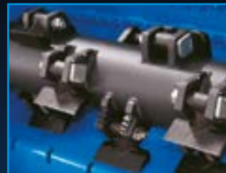
Rotore con supporti dentati Rotor with toothed supports
