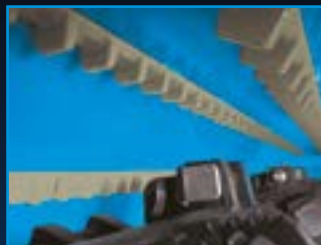
3 controcoltelli dentati 3 notched counter-knives
