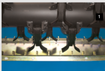
Contro-coltelli speciali a denti seghettati Special notched toothed counter-knives Contra-cuchillas especiales dentadas
