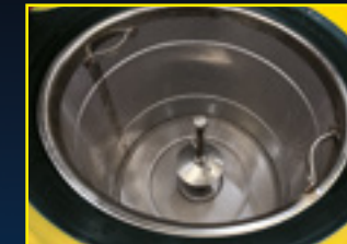
Cestello miscelatore e lavabottiglie in inox. Stainless steel mixing basket with bottle washer.
